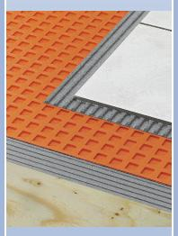
"We use Schluter Ditra, which provides a superior underlayment for floor tile installation," says Flyer. "By decoupling the stone from the wood beneath, this product helps to prevent movement and cracking of grout/tiles." The underlayment is also used on masonry and Terrazzo flooring applications.
