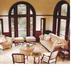
The fixed windows from Fenestra come standard in Mahogany with other timber options available and are available in any size or configuration. The company's waterproof adhesive is used on all joints, and the windows have simulated divided lites, applied brickmold casing and applied sub-sill. The glass is hurricane-impact and is IBC and SBCCI tested and rated.
